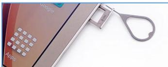
3. Insert Micro SD Card, label side up and ensure SD Card slot is closed properly.
