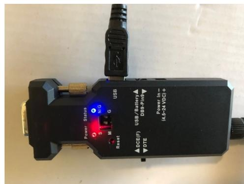
Make sure the sliding DCE/DTE switch on the side of the adaptor is set to DCE (F) and that the Power Source switch is set to USB/Battery.
